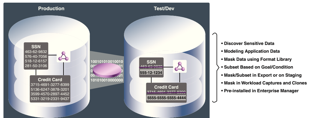
Figure 1-1 Oracle Data Masking and Subsetting Used in a Production and Test Database Setup
