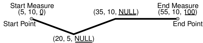
Figure 7-7 Creating a Geometric Segment
